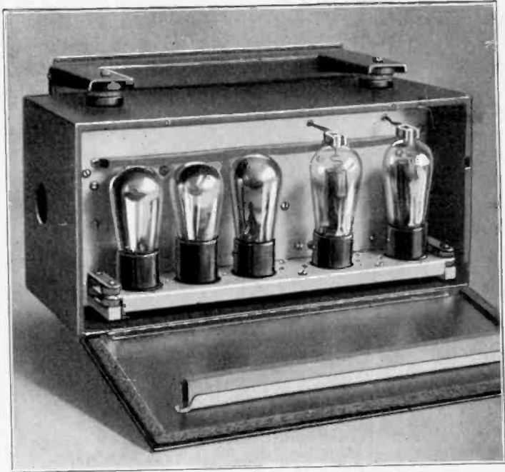
Fig. 5—Tube Compartment of Model B Receiver, Showing Shock Insulation of Tube Girder and Auxiliary Shock-Proof Support at Top of Tubes.
