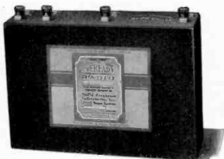
Fig. 4—Special Light-Weight Combined B and C Dry-Cell Battery for Use with Aircraft Receiver.
