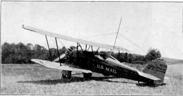
Fig. 1—Installation on Pitcairn PA-5 Mail Plane Showing Short Rigid Vertical Antenna.
