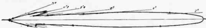
Fig. 5—Directivity of Grecian Curtain (Fig. 4) \lambda = 5.87 m. Symmetrical Left-hand Lobe of the Curve Has Been Omitted.
