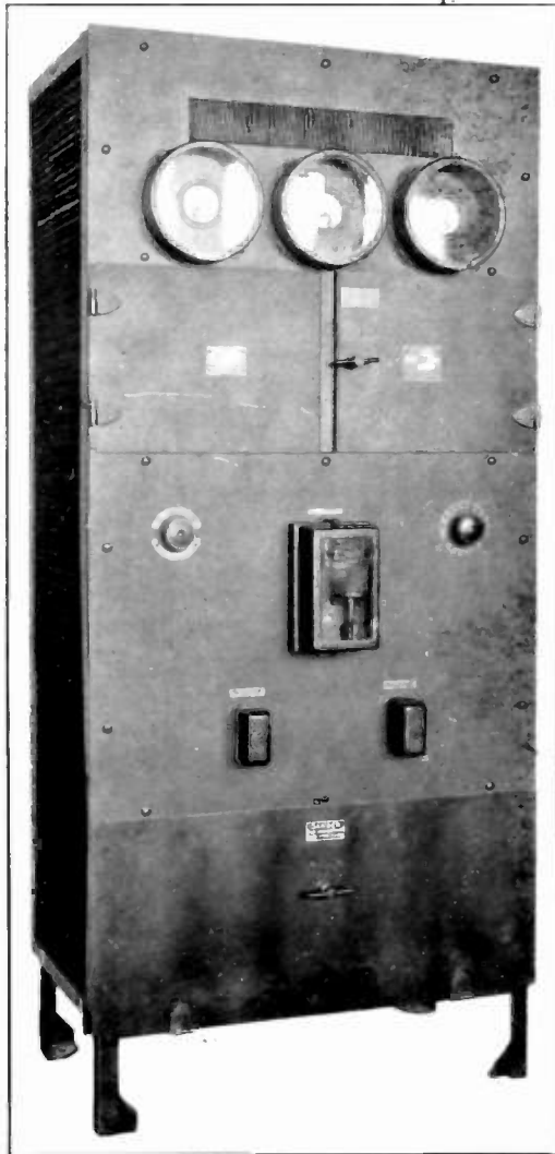
FIGURE 20—Transmitter Panel, Front
