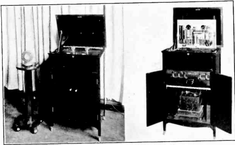
FIGURE 2—Condenser Transmitter Equipment
