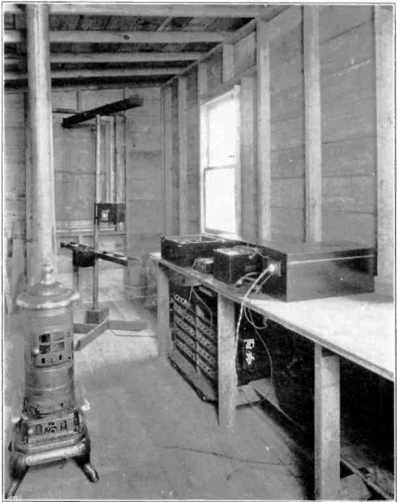
FIGURE 17—Short Wave Field Strength Measuring Set as Installed in the Measurement Shack at Cliffwood, New Jersey
