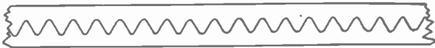
FIGURE 8—Record of Dashes at 60 Words per Minute on Cable Type of Siphon Recorder
