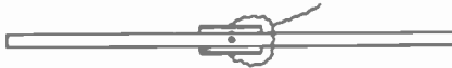
FIGURE 8—Steel resonator, the exciting quartz plates having tinfoil coatings electrically connected. The hook by which the steel rod is suspended serves as the other terminal
