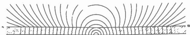
FIGURE 1—Suggested Distribution of Magnetic Field About a Submerged Cable Carrying Alternating Current
