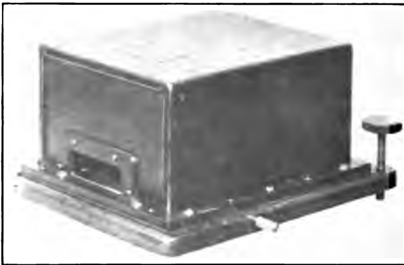
FIGURE 17—Galvanometer for Visual and Photographic Recorder (Associated View)
