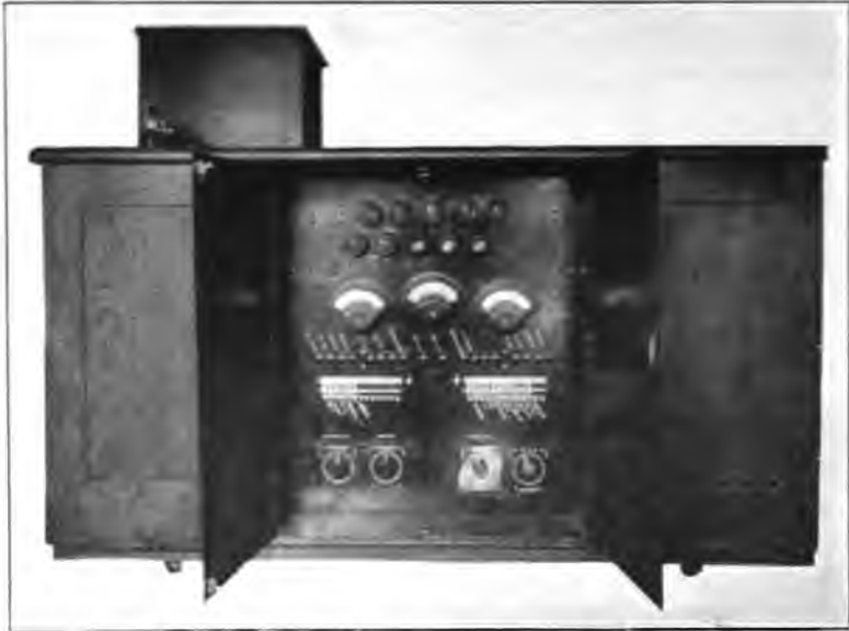
FIGURE 8—Rear View of Desk Showing the Battery Supply Panel
