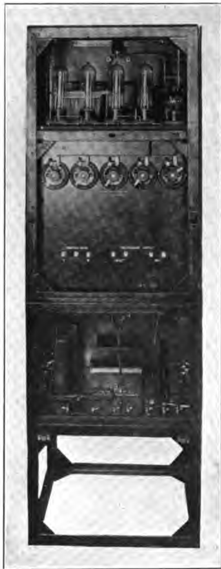
FIGURE 14—Radio Transmitter (Rear View)
