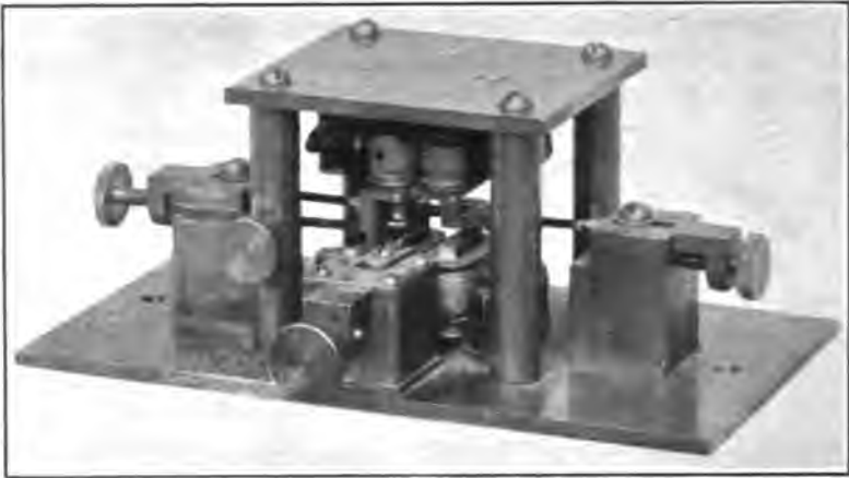
FIGURE 1—First Model of Galvanometer for Visual Reception
