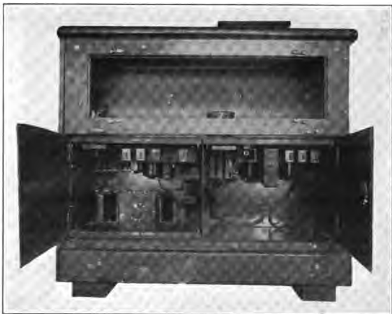
FIGURE 7—View of the End of the Repeater Desk
