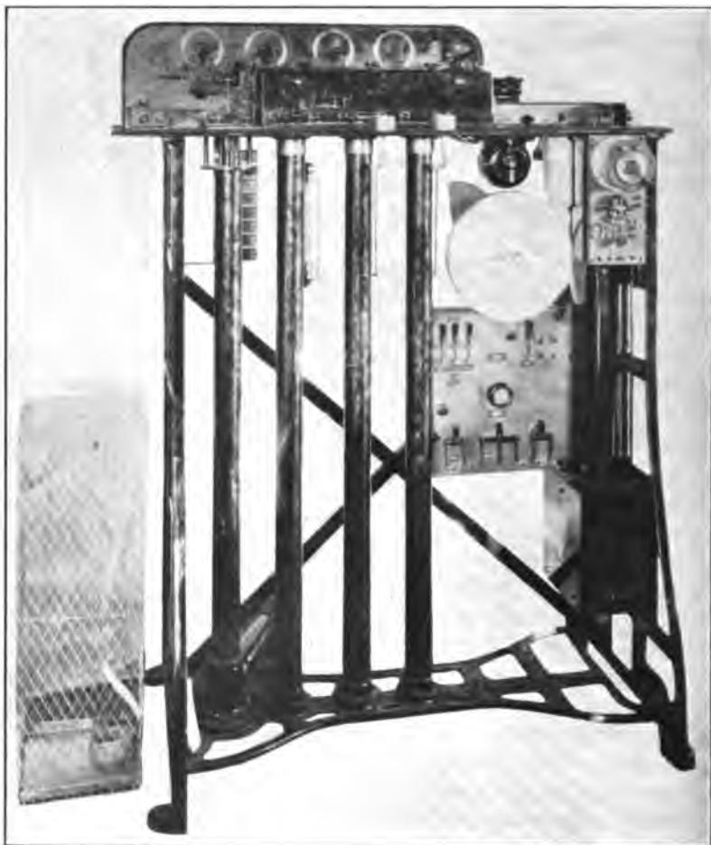
FIGURE 12—Visual and Photographic Receiving Device—Front View
