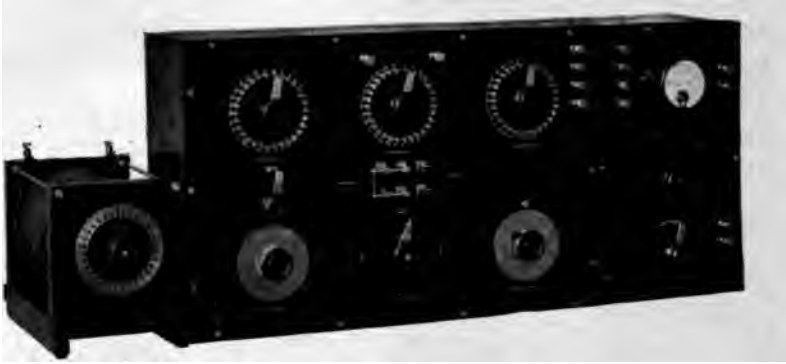
FIGURE 6—Bridge Receiving Set for Duplex Radio Telegraphy
