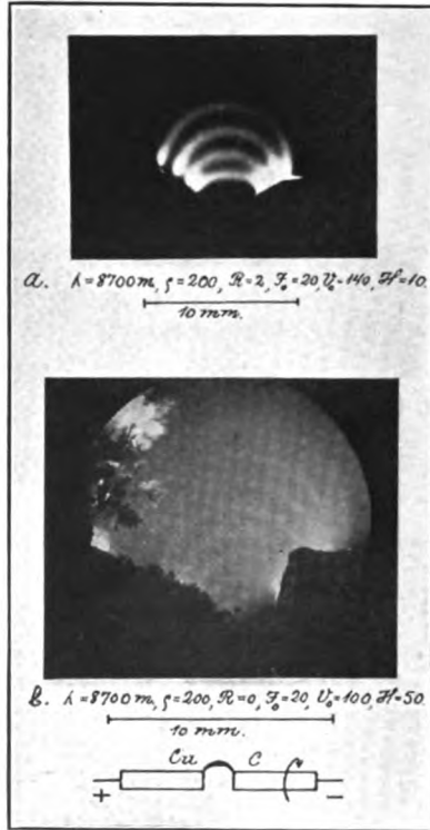
FIGURE 19a—Side Views of Arcs in Weak Fields. Part A in Hydrogen. Part C in Coal Gas
