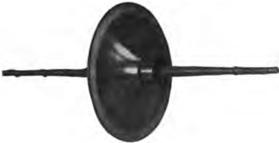
FIGURE 2—Rotor and Shaft of Standard 100,000-Cycle Alternator
