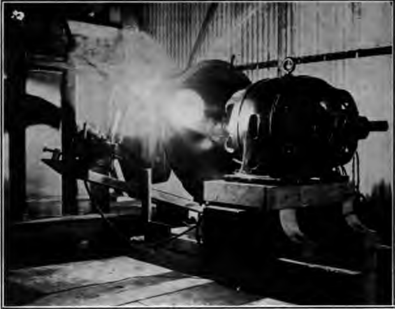
FIGURE 7—25 K.W. spark; note synchronism of disc indicated by the stud near top of disc. Exposure 20 seconds during which time disc made 597 revolutions. Ketchikan
