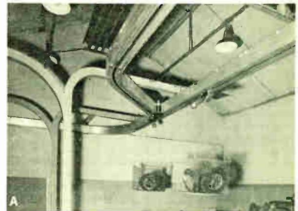
FIGURE 38. A—General view of the Linerail. B—Close-up of truck that runs within the girder. The top portion contains the primary of the motor, with the upper part of the girder as secondary and the air gap kept constant by four small rollers. Collecting brushes are seen to the right, with four main wheels to support the load on the bottom (it should be noted that the motor is vertically independent of the remainder of the truck).
