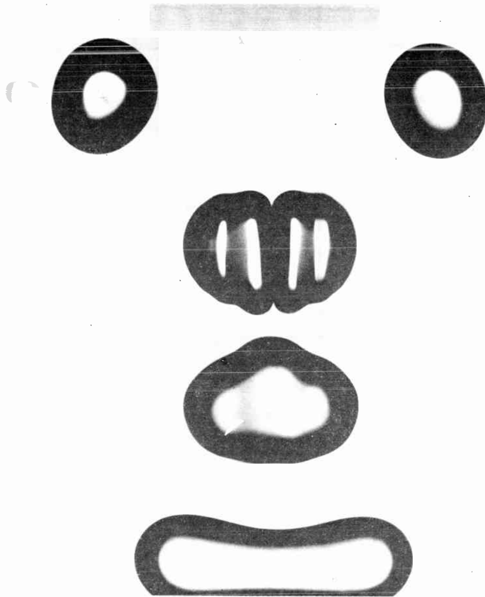
FIGURE 1. Water droplets that first condense from the vapor state to form clouds in nature are only a few micrometers in diameter, far too small to fall as rain. Collisions like the one you see taking place in this laboratory experiment help them to coalesce into larger drops that can reach the ground. In this experiment, one of a continuing series being carried out under the direction of J. Doyne Sartor at the National Center for Atmospheric Research, two streams of water droplets, each 780 \mu\text{m} in diameter and separated from the next by a time interval of 50–100 \mu\text{s} , were projected toward each other from the upper left and upper right. Only the leading droplets in each stream are visible in this photograph. Successive droplet pairs collided and coalesced with monotonous regularity—as you can see—because droplet trajectories, inertias, and interaction times could be manipulated mechanically to achieve this result. To achieve comparable results in clouds, however, and thereby to produce or prevent rain, it may be necessary to manipulate the charges carried by cloud droplets, or the electric field within the cloud, because electrostatic attractive forces contribute significantly to most collisions that lead to coalescence in the early stages of precipitation particle growth. This alternative to conventional cloud seeding has been explored by several groups in the past few years.
