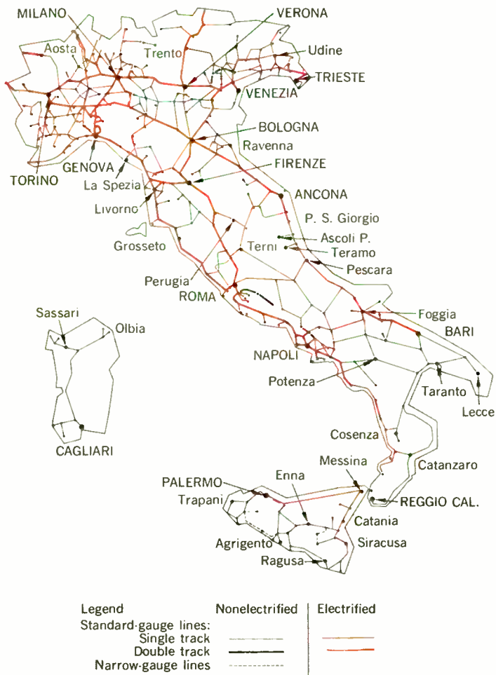
FIGURE 13. Map showing the extent of the Italian State Railways' electrified network as of January 1, 1965.
