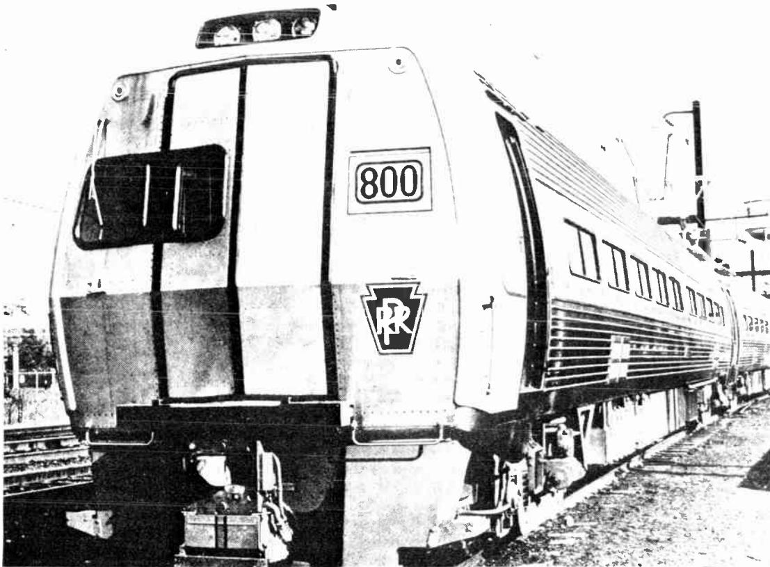
FIGURE 7. Streamlined front-end view of two of the new permanently coupled "Metroliner" high-speed multiple units soon to be placed in service on the Washington–New York run.
