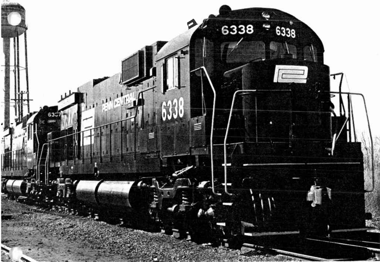
FIGURE 1. Two modern Penn Central diesel-electric road and switching locomotives coupled together for operation as a multiple unit by engineman in the front cab.
