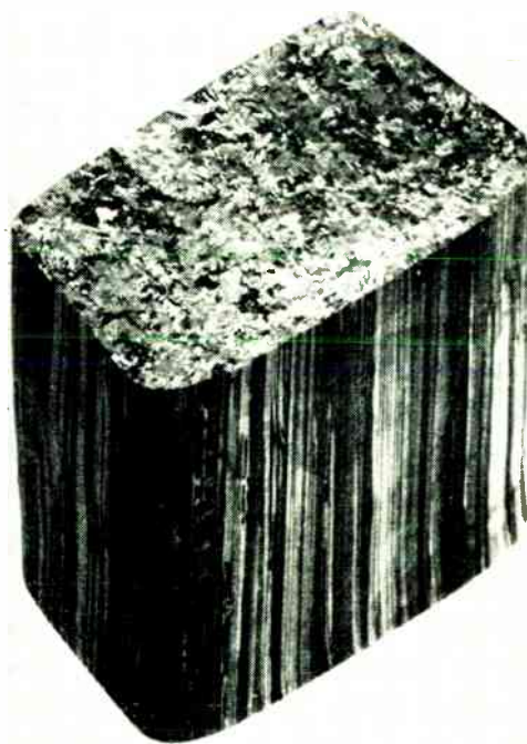
FIGURE 13. Fiber crystal of InSb-NiSb with the single thin elongated crystals oriented in the \langle 110 \rangle -direction.
