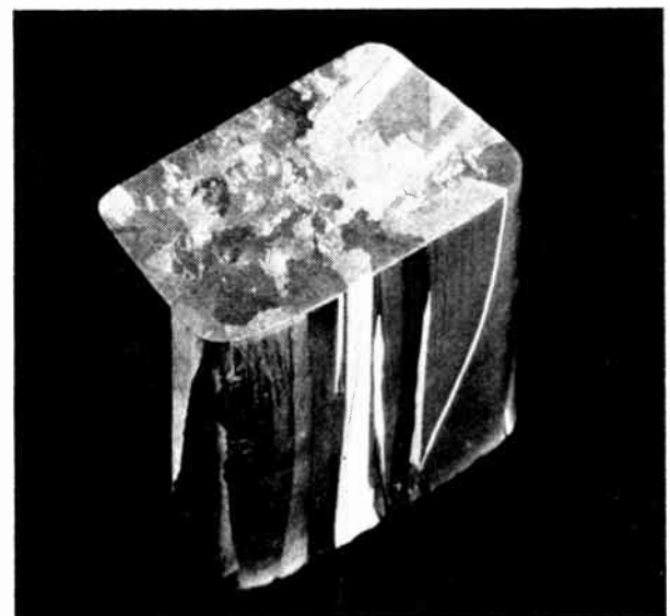
FIGURE 11. Polycrystalline rod of InSb-NiSb. This cross-sectional area is 2.5 cm \times 2 cm.
