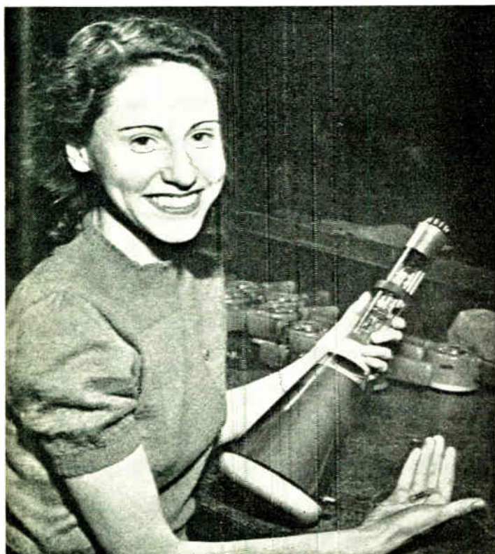
FIGURE 7. Electronics technician holds a conventional 5-inch cathode-ray oscilloscope tube and a subminiature radio tube of the type used in the proximity fuze.
