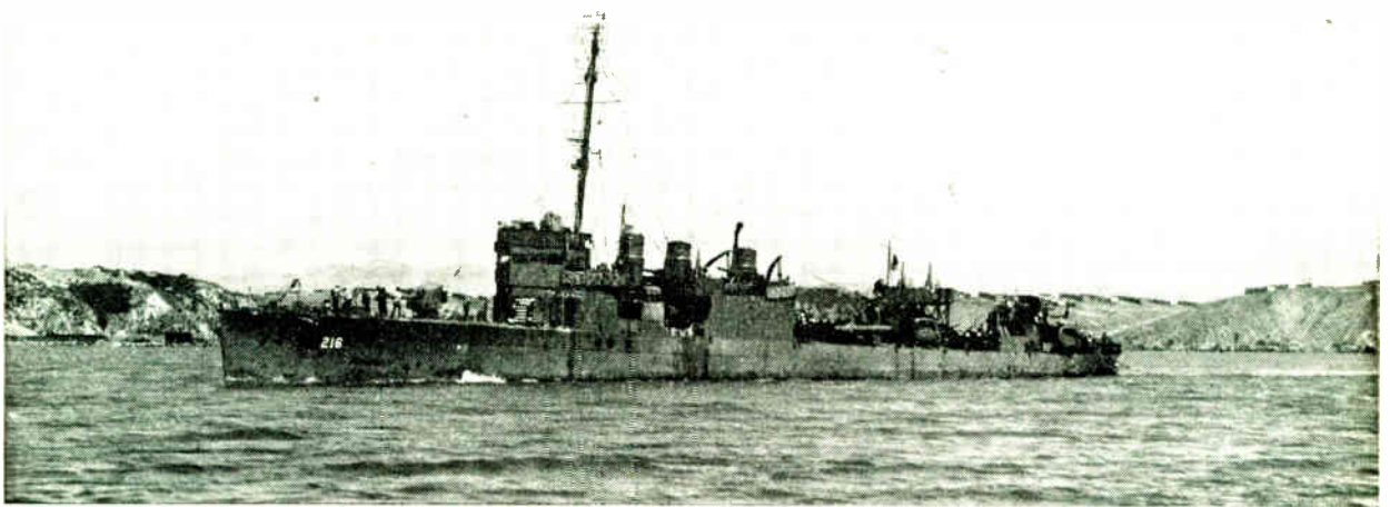
FIGURE 1. The World War I-vintage flush-deck destroyer U.S.S. John D. Edwards (DD-216), a veteran of the Battle of the Java Sea, shown at Mare Island Navy Yard on 9 September 1942, after extensive repairs and refitting. Note the “bedspring”-type radar antenna on the foremast.
