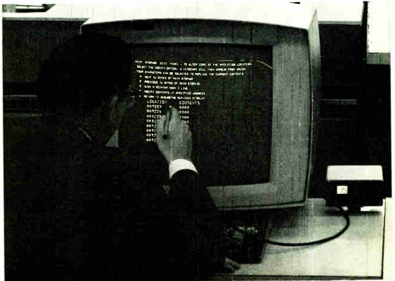
FIGURE 4. The IBM 2250 graphic data-processing system
