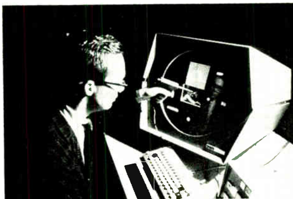
FIGURE 2. The digital cathode-ray display console allows experimental operations on many different types of function formats.
