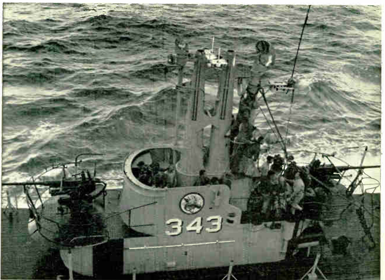
FIGURE 13. Air-search and surface-beamed rotating radar antennas aboard the submarine U.S.S. Clamagore (SS-343). Many metallurgical, mechanical, and electrical problems had to be overcome before reliability of this apparatus, subject to long periods of immersion, was assured.
