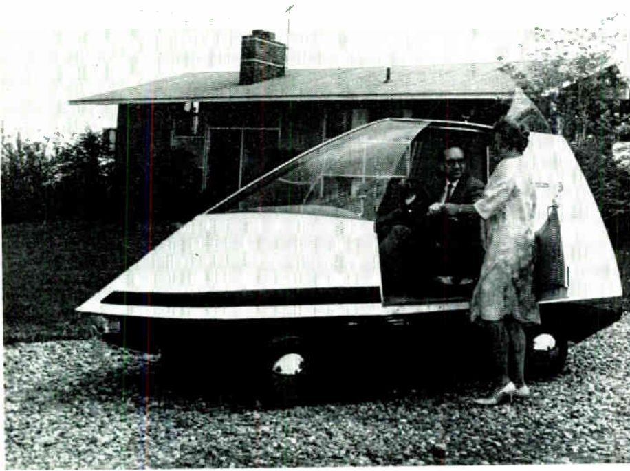
FIGURE 7. The so-called staRRcar represents an innovation in transportation. These small electric vehicles would carry people around, on wheels and on guideways, in a combination of private and public transit. A somewhat similar system, in which the vehicles would be owned and maintained by a transit authority, was proposed by Dr. Richard C. Dorf, University of Santa Clara, at an electric automobile symposium, held in February 1967 at San Jose State College, California.
