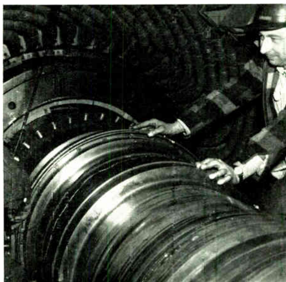
Fig. 12. Overall view of Con Edison's 1000-MW Ravenswood no. 3 generating unit. This cross-compound machine is the largest in the world. It began supplying the system on June 7, 1965.
