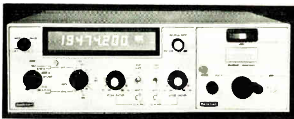
Fig. 6. Type NU58A multinumeric, as employed on a Beckman Instruments Corporation frequency counter.
