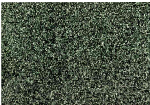
Fig. 3. Duplication of Oliver's photograph, except that transmission rather than scattering diffraction is used. (Difference in grain size is caused by dissimilar degree of enlargement)
