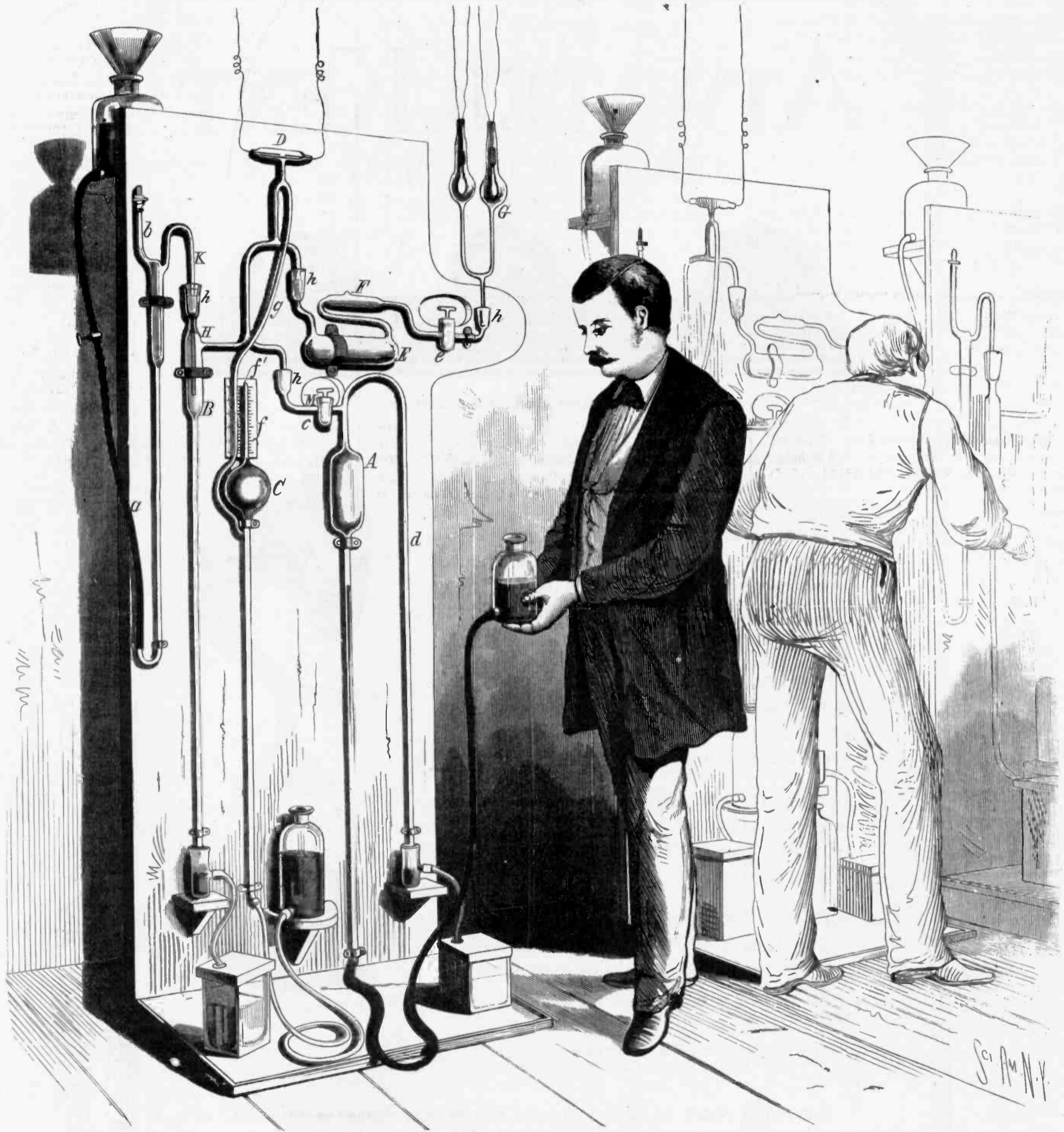
A.—Geissler's Pump. B.—Sprengel's Pump. C.—McLeod's Gauge. D.—Geissler Tube. E.—Bulb containing Phosphorous Anhydride. F.—Bulb containing Gold Leaf. G.—Electric Lamp Bulbs. a.—Mercury Supply Tube. b.—Air Trap. c. and e.—Mercury Sealed Stop Cocks. d.—Discharge Tube. f.—Scale. f'.—Gauge Tube. g.—Connecting Tube. h.—Mercury Sealed Joints.
