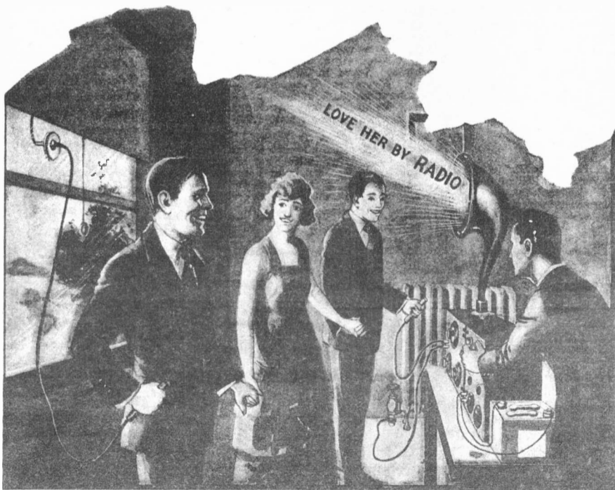
To Demonstrate the Intensifying Power of Modern Vacuum Tube Receivers, It Is Interesting to Show How Several People May Be Placed in Series With the Antenna Wire and the Receiving Set, as Here Shown. The Radio Current Picked Up by the Antenna Will Pass Thru the High Resistance of the One or More Persons, and the Signals Will Be Heard in the Receiving Set Just the Same. This Experiment Was Performed Quite Early in Radio History by Dr. Marconi Himself.
