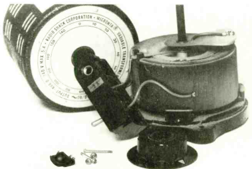
The autotransformer is a one-coil device wound on a cylindrical iron form with the AC line connected across the bottom of the coil and to a tap on a copper turn about 85% of the distance from the first tap. A sliding contact selects one of the coils to pick off an AC voltage. The plastic piece hanging from the leads of the winding was discarded because it was damaged and the single outlet was neither polarized nor of the three-terminal type.
