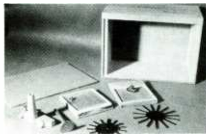
This is the preliminary stage in the construction of Dan Damrow's Crosley 50 replica. The fabricated parts for the coils and "book" condenser are in the foreground.
