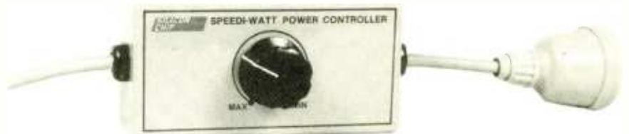
This is what Speedi-Watt looks like when it's finished. The neat all-plastic construction ensures against possible shock hazard.
