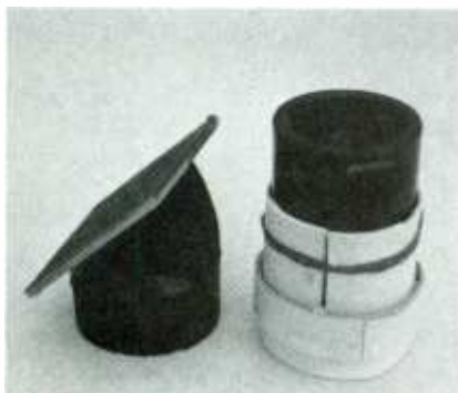
A mirror mounted atop the cardboard tube at a 45 degree angle and fitted over the projection lens allows the kaleidoscope images to be projected on a wall screen.
