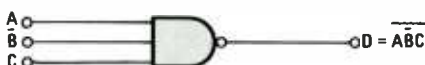
Fig. 10. In a NAND expression, the result of all ANDing is simply inverted.
