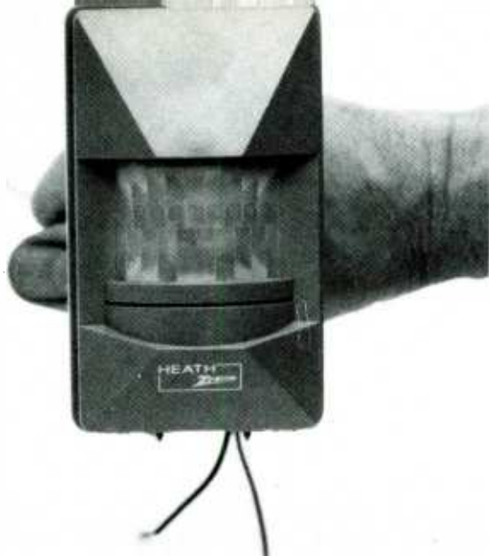
The SL-5410 Entryway Light Control, like other sensor modules in the SSA-5910 Security System, is capable of detecting heat given off by moving objects. When someone enters its sphere of detection, the SL-5410 can switch on up to a 500-watts of lighting. It also has a built-in light sensor, which turns the lighting off during the day-light hours.
