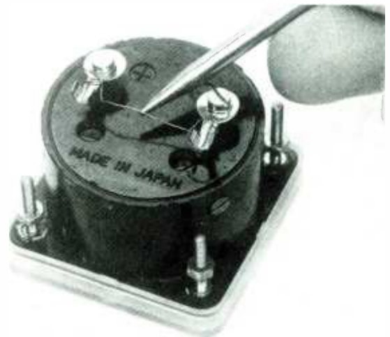
Fig. 6—Your meter will most likely come with a shorting wire across its terminals. Leave the wire in place until the FSM is completely assembled. Then cut the wire free.
