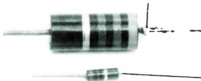
Fig. 4—The large 2-watt carbon resistor at the top is the coil form for L1. The ¼-watt resistor at the bottom is shown just for size comparison.
