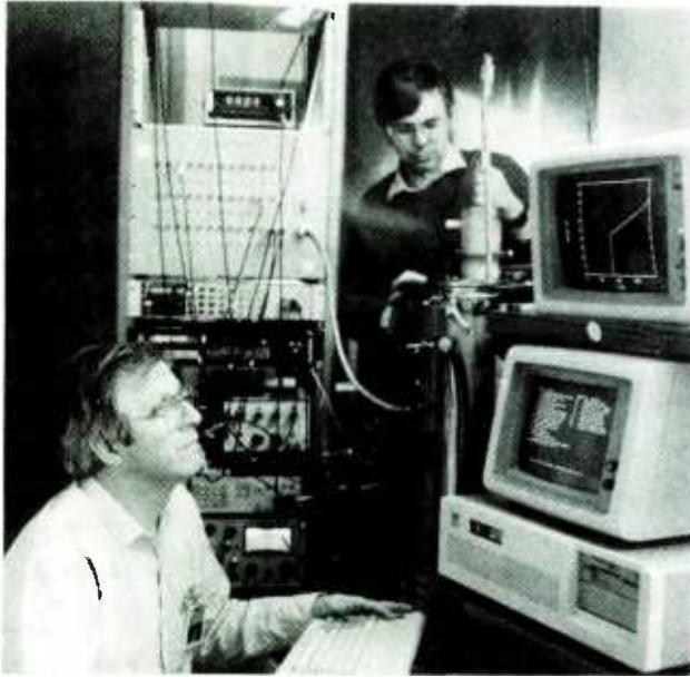
IBM scientists are measuring a superconducting material. The graph on the upper monitor shows the sudden drop in electrical resistance of the material as its temperature drops below the superconductivity transition temperature after immersion in liquid nitrogen. (Photo courtesy of IBM.)
