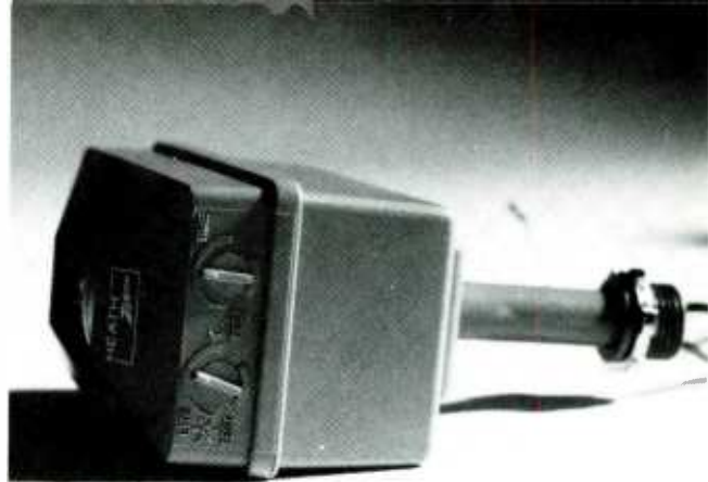
The SL-5410 Entryway Light Control, like other sensor modules in the SSA-5910 Security System, is capable of detecting heat given off by moving objects. When someone enters its sphere of detection, the SL-5410 can switch on up to a 500-watts of lighting. It also has a built-in light sensor, which turns the lighting off during the day-light hours.
