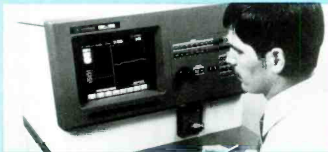
Here's HYPRES' PSP-1000 Picosecond Signal Processor. It can actually handle picosecond signals, unheard of in transistor technology. (Photo courtesy of HYPRES, Inc.)
