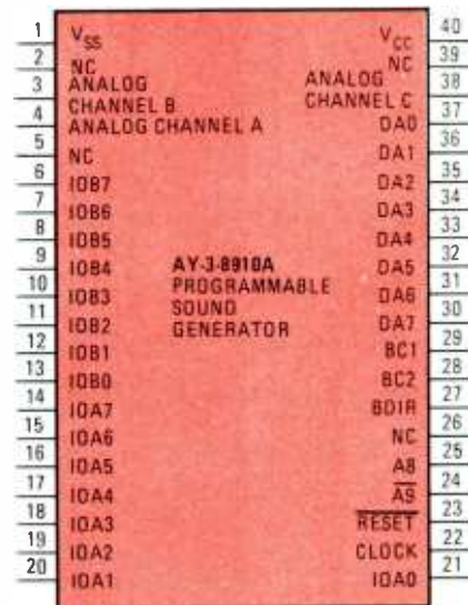
Fig. 1—Shown here is a block pinout diagram of the AY-38910A programmable sound generator. To take full advantage of the PSG’s capabilities requires a computer with 8 bidirectional data lines, 2-control lines, and 1 line to zero the registers. Data loaded into its 14 bidirectional registers controls tone pitch, noise pitch, channel volume, and amplitude modulation.
