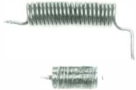
Fig. 5—This is how the two coils should look when ready for installation. Make sure you tin their ends with solder before installing the coils.
