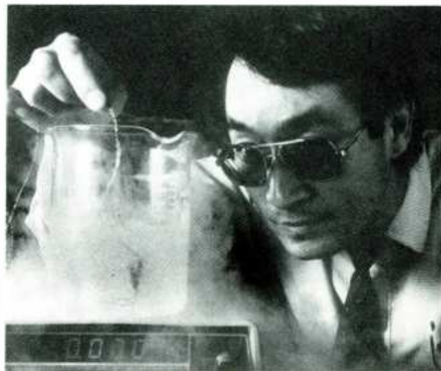
A team of scientists at AT&T Bell Laboratories has succeeded in developing superconducting wires that can easily be formed into coils. Shown here, the superconducting wire is being immersed in liquid nitrogen. The wire is clad in a metal coating for electrical, thermal, mechanical, and environmental protection. (Photo courtesy of AT&T Bell Laboratories.)
