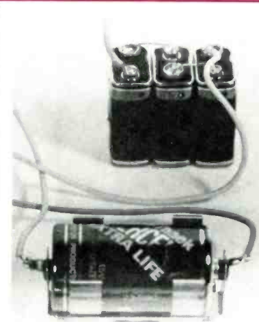
Powering up the little set required only three 9-volt transistor radio batteries wired in series and a D-size flashlight cell.
