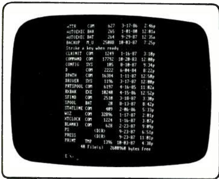
Fig. 1—This is how your directory listing will look when you enter DIR/P. Only part of the directly is available.
