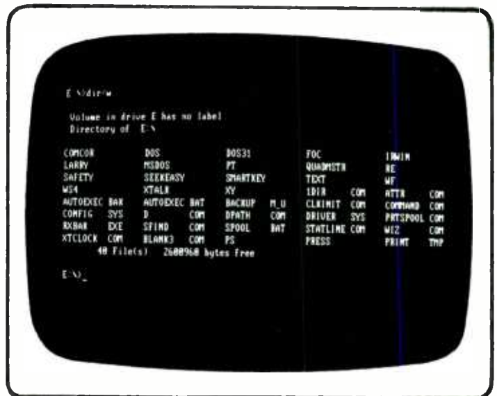
Fig. 2—Here's the same directory as in Fig. 1 but using the DIR/W command. Time, date, and size have been stripped.
