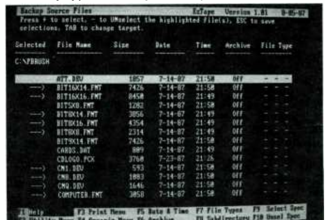
Next you choose the files one by one or by group. Here we first selected all files, and then de-selected several for demonstration purposes. Using F9 and F10 you can select files by name, using wildcard characters ( * and ? ).
