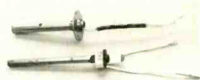
Actually, the tip's business end is really a hollow heating element (top) and switch that slides into the element.
