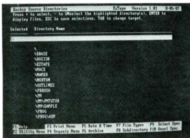
After choosing "Select files and backup" from the previous menu, you are presented with a list of subdirectories, which can be selected all at once or one by one.
