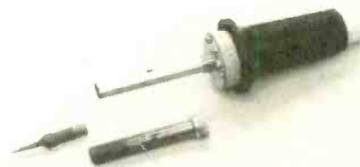
The business end of a soldering station's handle looks simple enough. A heating element, a replaceable soldering tip, and a sleeve that holds the tip in place. Circle no. 77 on the Free Information Card.
