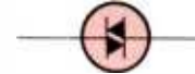
Fig. 12— Since a device such as a triac requires trigger signals during either half-cycle the AC waveform the diac was invented to permit a pulse to pass in either direction.
