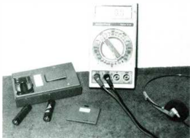
Check those batteries when the radio becomes weak, dead, or distorted. It's a good idea to check the voltage of each battery while the radio is operating. A battery tester may be used.
