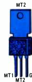
Fig. 20—Note that MT2 is also the heat sink and should be the lead connected to the ground plane to avoid shorts.
