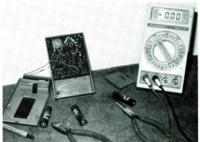
Inspect the printed-circuit board for damage if the radio was dropped. Use the pencil eraser to prod or move the various components. Intermittent reception may be caused with cracked resistors, broken connections, and poor solder connections.
