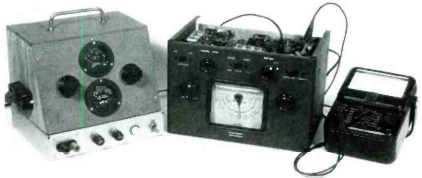
The Start-Up Console (outlined in the August 1987 column) was used to gradually raise EC-1's AC supply voltage during the initial start up. A multimeter was used to monitor the set's plate voltages.
