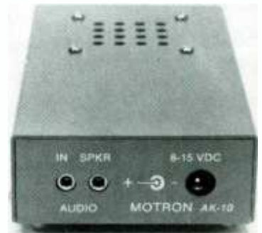
The rear has connections for the DC power supply, input from the receiver, and a switched output for a speaker.
