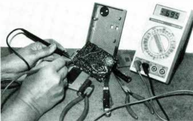
Quickly check each transistor in the audio-output stages with the DMM's diode-test mode for leakage when sound is distorted. Usually, a couple of small screws hold the radio chassis to the case. Mark each transistor terminal for easy replacement.
