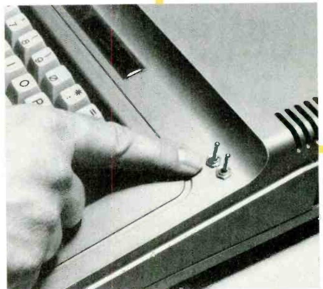
Mounting the switches on the front panel, rather than the rear, makes them convenient to use. However, if you need to remove the cover in the future, you'll have to remove the switches.
