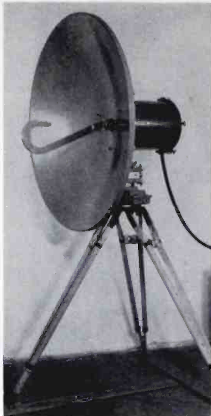
FIG. 6. AN RCA MOBILE MICROWAVE LINK UNIT. THE TRANSMITTER IS IN CYLINDRICAL HOUSING
