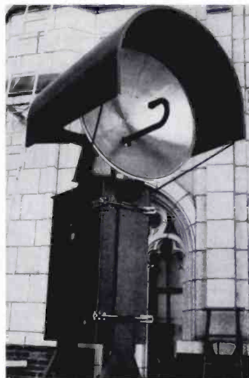
FIG. 5. TWO VIEWS OF A MOTOROLA 7,000-MC. TRANSMITTER-RECEIVER-ANTENNA COMBINATION UNIT
