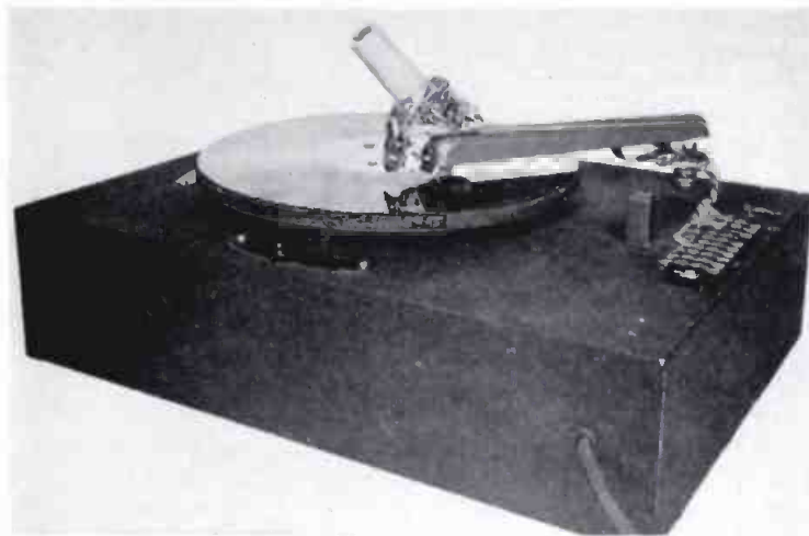
FIG. 1. DISTORTION OF SINE WAVE BY LONGITUDINALLY COMPLIANT STYLUS. FIG. 2. APPARATUS FOR MEASURING LONGITUDINAL STYLUS EXCURSION
