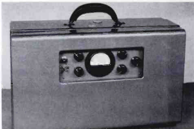
FIG. 7. RCA MICROWAVE TRANSMITTER CONTROL UNIT. FIG. 8. RECEIVER CHASSIS, DESIGNED SAME WAY AS TRANSMITTER, WITH SIMILAR CONTROL UNIT
