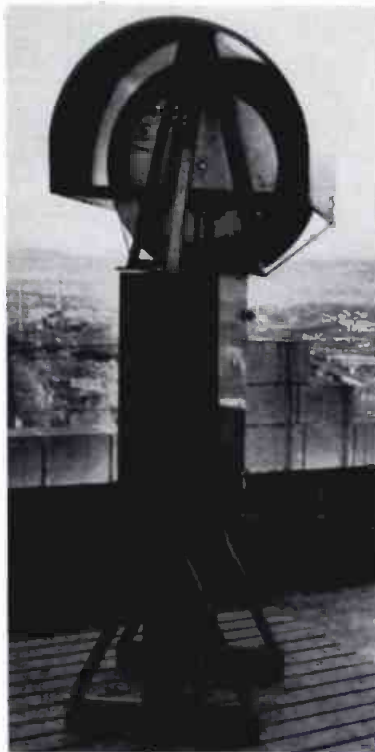
FIG. 5. TWO VIEWS OF A MOTOROLA 7,000-MC. TRANSMITTER-RECEIVER-ANTENNA COMBINATION UNIT
