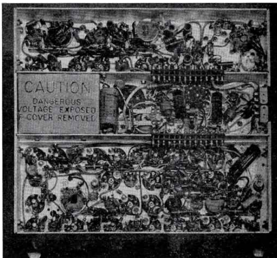
FIGS. 3 AND 4. TOP AND BOTTOM OF COMBINED TRANSMITTER, RECEIVER, AND VIBRATOR POWER-SUPPLY CHASSIS. NOTE SINGLE-LEVEL PARTS MOUNTING
