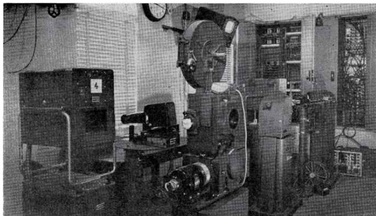
FIG. 4. FILM AND SLIDE EQUIPMENT, INCLUDING 35-MM. PROJECTOR AND ICONOSCOPE FILM CAMERAS
