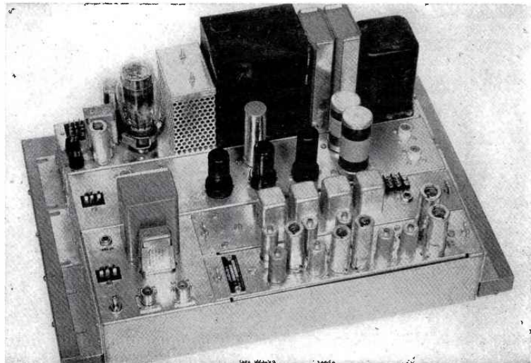
FIG. 4. SUBCARRIER RECEIVER AND FILTER, MOUNTED EXTERNALLY WITH VIDEO OUTPUT AMPLIFIER
