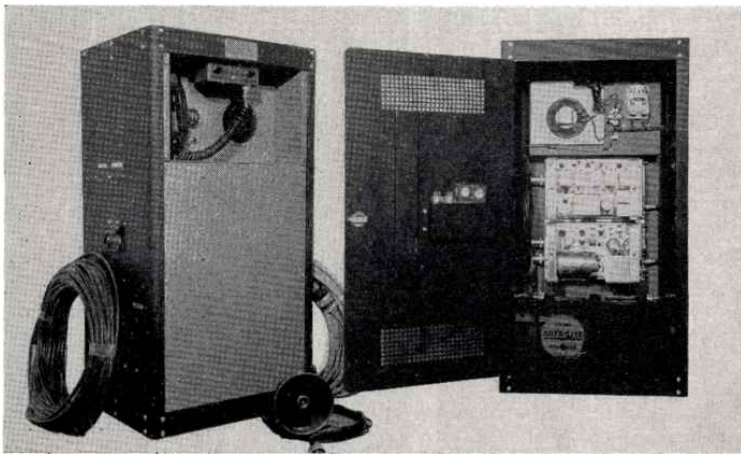
WHEN INSTALLATIONS IN THE OIL FIELDS REQUIRE 6-VOLT OPERATION, COMMUNICATIONS ENGINEERING COMPANY OF DALLAS USES G.E. MOBILE UNITS, ASSEMBLING THEM IN THIS MANNER
