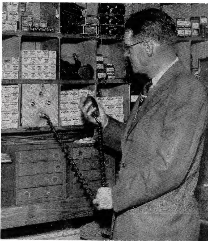
FIG. 2. TO CHECK THE MICROPHONE CIRCUITS, CORD IS PLUGGED INTO THE TESTER AND FLEXED
