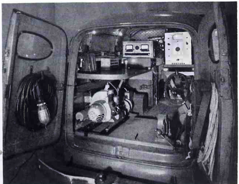
FIG. 12. THE 4-WHEEL DRIVE VEHICLE FOR MAINTENANCE AND SUPPLY RUNS TO REPEATERS. FIG. 13. FIELD SERVICE TRUCK HAS PORTABLE GENERATOR
