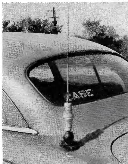
FIG. 2. THE SPRING-AND-SWIVEL BASE MOUNT
