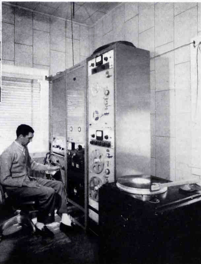
FIG. 4. OPERATOR-ANNOUNCER LINDY SEAMON AT THE STUDIO CONSOLE FACING THE TRANSMITTER ROOM. FIG. 5. ANTENNAS FOR THE ORDER CIRCUIT AND THE S-T LINK. FIG. 6. ENGINEER-OPERATOR RALPH THOMPSON AT THE RACKS WHICH CARRY THE AUDIO EQUIPMENT, RELAY FM RELAY RECEIVER AND THE S-T LINK RECEIVER AND DUAL PRESTO TAPE RECORDERS
