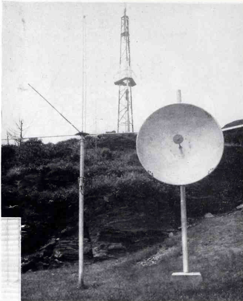
FIG. 4. OPERATOR-ANNOUNCER LINDY SEAMON AT THE STUDIO CONSOLE FACING THE TRANSMITTER ROOM. FIG. 5. ANTENNAS FOR THE ORDER CIRCUIT AND THE S-T LINK. FIG. 6. ENGINEER-OPERATOR RALPH THOMPSON AT THE RACKS WHICH CARRY THE AUDIO EQUIPMENT, RELAY FM RELAY RECEIVER AND THE S-T LINK RECEIVER AND DUAL PRESTO TAPE RECORDERS
