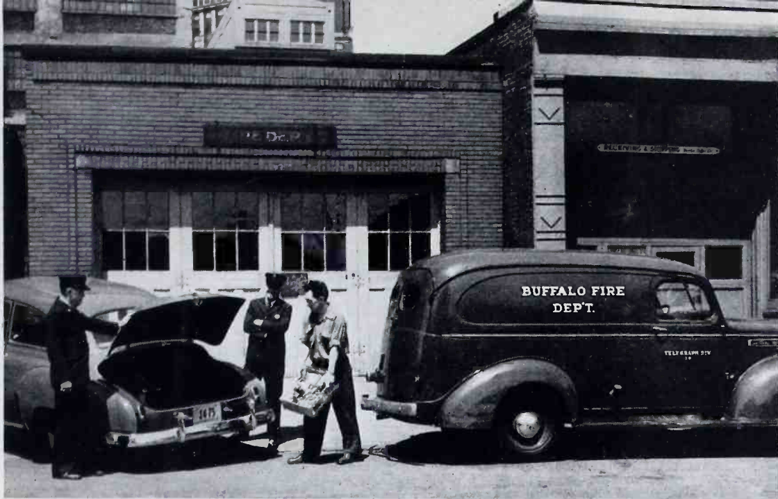
FIG. 10. RADIO SERVICE TRUCK IS USED FOR EMERGENCY REPAIRS, AND AS A FIELD RADIO STATION
