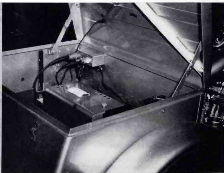
FIG. 2. RADIO AND SELECTIVE CALLING CONTROLS, AND MOUNTING FOR THE HANDPIECE. FIG. 3. INSTALLATION OF THE COMPLETE RADIO EQUIPMENT
