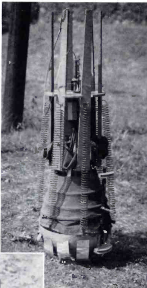
FIG. 1, ABOVE: THE GRASSHOPPER AS IT APPEARS WHEN IT LANDS, AFTER THE FIRST EXPLOSIVE CHARGE HAS THROWN OFF THE PARACHUTE. IF IT DOES NOT LAND UPRIGHT, THE SIX LEGS BRING IT TO AN UPRIGHT POSITION
