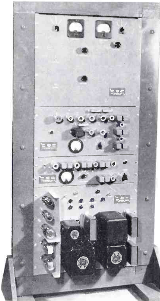
FIGS. 4, 5, 6. FRONT AND TWO REAR VIEWS OF THE 900-MC. TRANSMITTER FOR USE WITH STANDARD TELEPHONE CHANNELIZING EQUIPMENT
