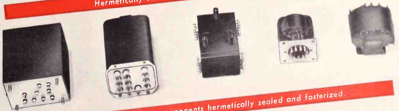
Hermetically sealed audio and pulse transformers.
