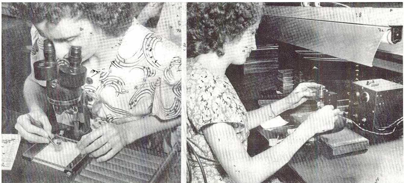
Fig. 4. A binocular microscope is used at each assembly stage. Fig. 5. This girl is checking grids with a contact micrometer.
