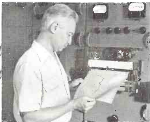
Automatic recorder plots sound pressures developed in the ear canal at different frequencies.
