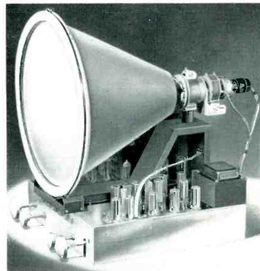
Fig. 1. Mounting takes 16- or 19-in. tubes
