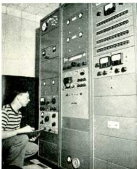
FIG. 13. Standard equipment includes, left, meteorological instruments and noise and distortion analyzing units; center, relay receivers and nemo receivers; right, amplifier and monitor. FIG. 14. Antenna for ST transmitter. FIG. 15. ST transmitter
