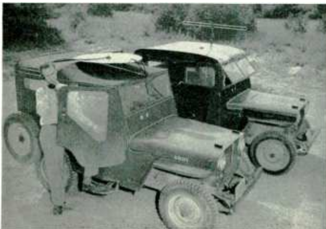
FIG. 3. Types of antennas installed on our Jeeps. FIG. 4. Speaker was mounted on the dash, with transmitter-receiver at the right
