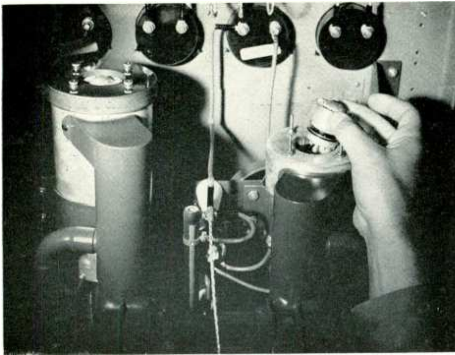
FIG. 2. Type 4X150A tripler and doubler stages deliver 15 watts at 940 to 952 mc.
