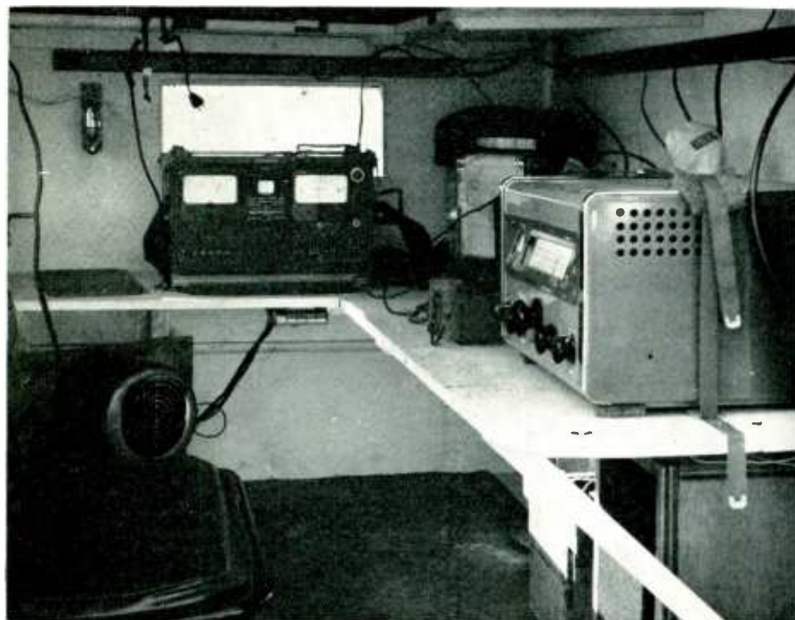
FIG. 2. Interior of mobile laboratory, showing field-strength measuring equipment
