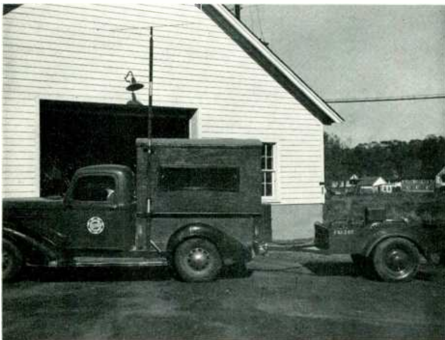
FIG. 1. The mobile laboratory used for the preliminary field strength surveys
