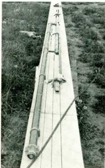
FIG. 6. Transmission-line harness for four bottom sections.
