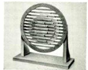
Laboratory model of the new lens. A similar arrangement of metal strips is concealed in the foam plastic blocks in the large picture.
