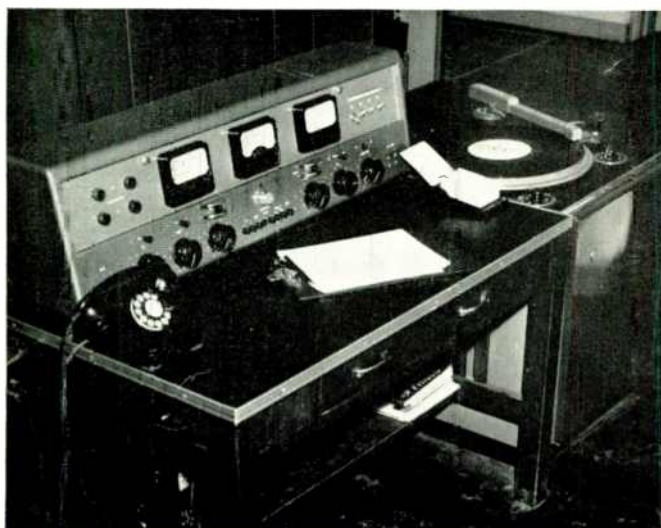
Fig. 10. FM transmitter control and monitor. Fig. 11. Shading console for film projector, and TV control and monitor right
