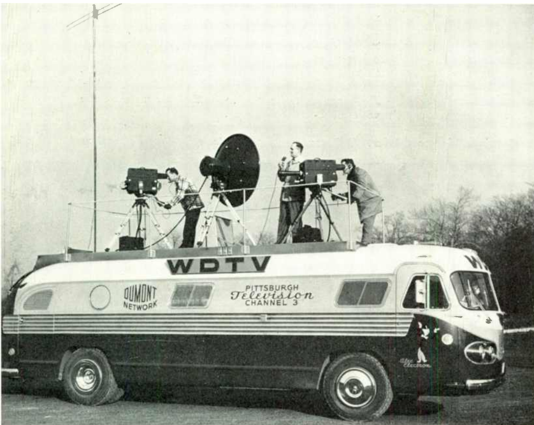
Fig. 1. Mobile studio set up for an outdoor program. Dipole is for station monitor
