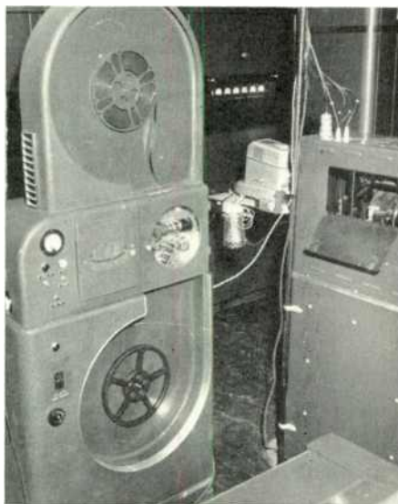
Fig. 3. The 16-mm. projector, left; slide projector, center; kinescope at right
