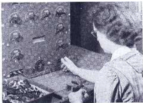
Every carbon element that goes into Mallory controls is individually inspected to be sure that its resistance value is the same as specified on the labels.
