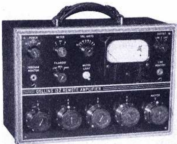
FIG. 8. 4-CHANNEL REMOTE PICKUP AMPLIFIER FOR AC OR BATTERIES. FIG. 10. 2-CHANNEL UNIT, WITH MIXER AND VU METER
