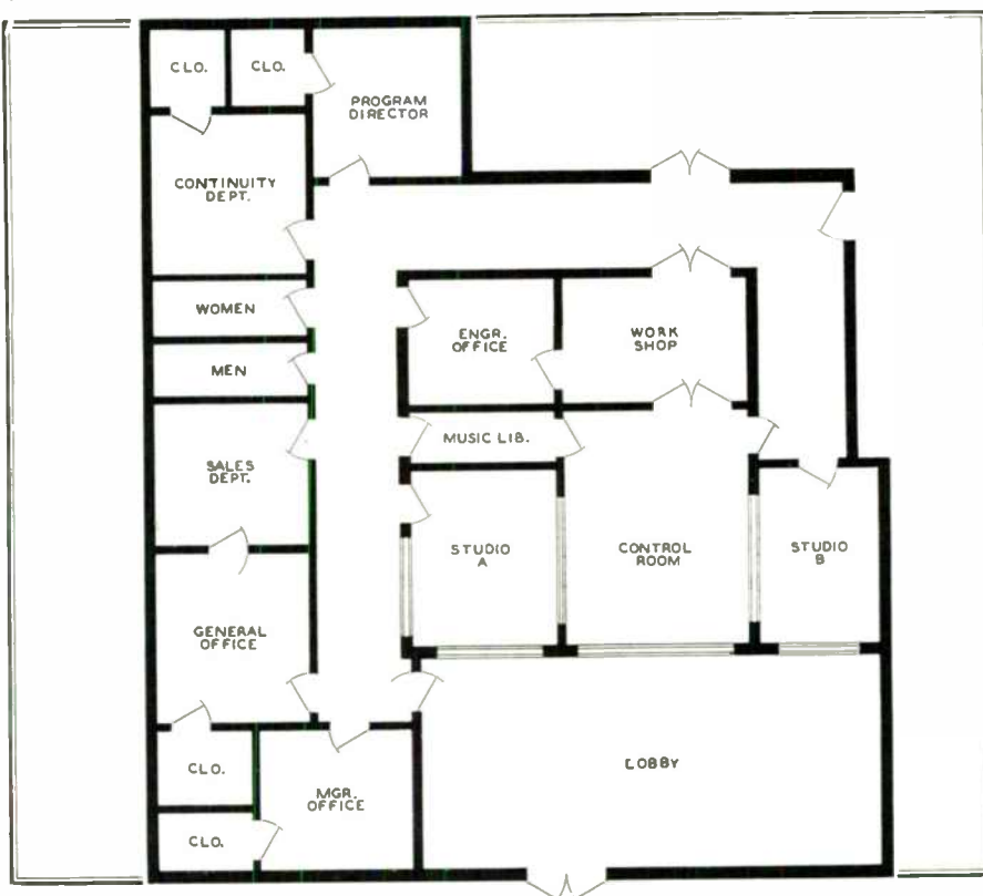
FIG. 1. THE FACILITIES SHOWN IN FIG. 2 ARE PLANNED FOR OFFICES AND STUDIOS SIMILAR TO THE LAYOUT SHOWN HERE FOR A SMALL FM OR AM INSTALLATION
