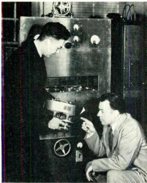
FIG. 1, ABOVE: JACK MCCULLOUGH, LEFT, AND BILL EITEL, WITH ONE OF THE NEW 3X12500A3 TRIODES. BELOW: 6-BAY TURNSTILE ON THE EIMAC PLANT AT SAN BRUNO, NOW SET UP FOR TEMPORARY USE
