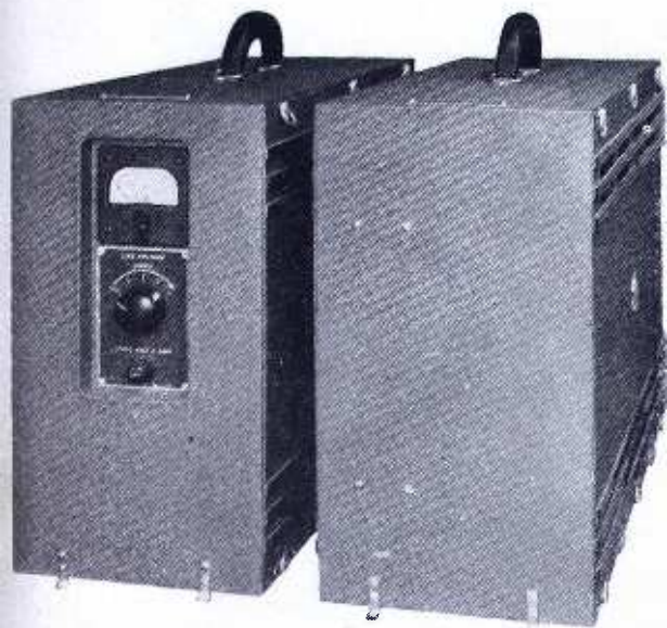
FIG. 18. PULSE-FORMING UNIT, LEFT, AND PULSE-SHAPING FIELD UNITS
