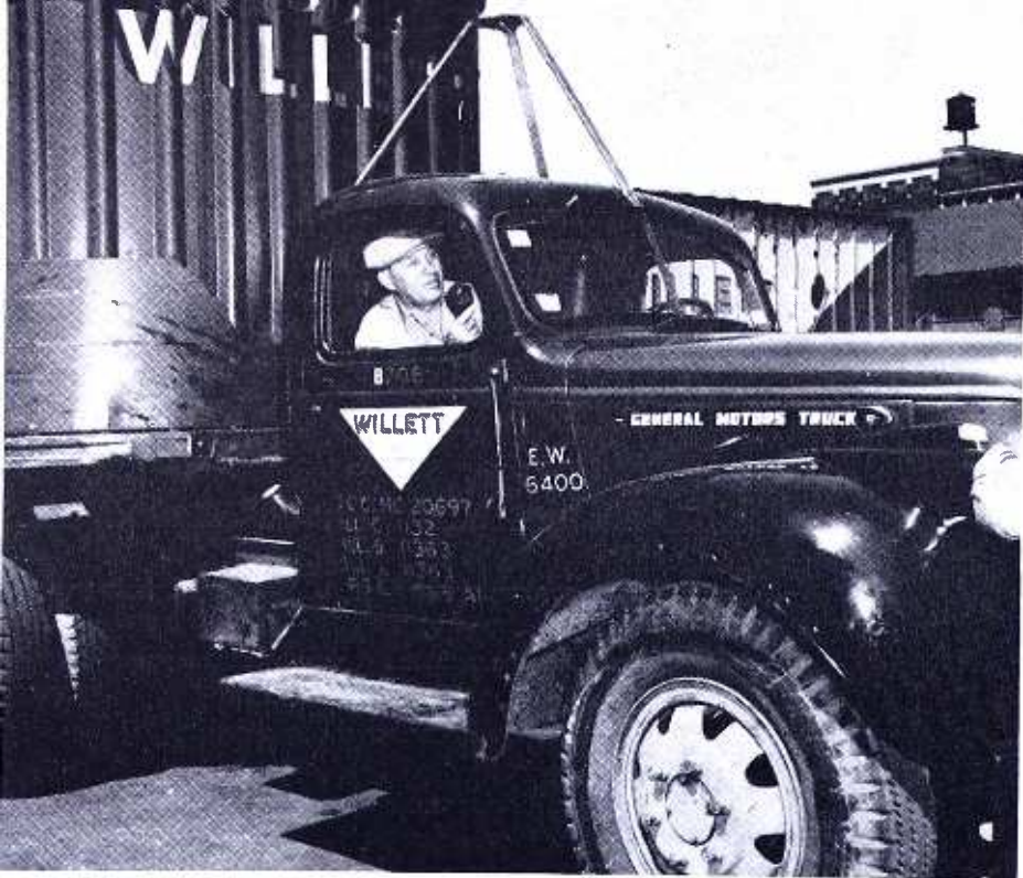
FIG. 1. TYPICAL ANTENNA MOUNTING ON A POWER UNIT.
