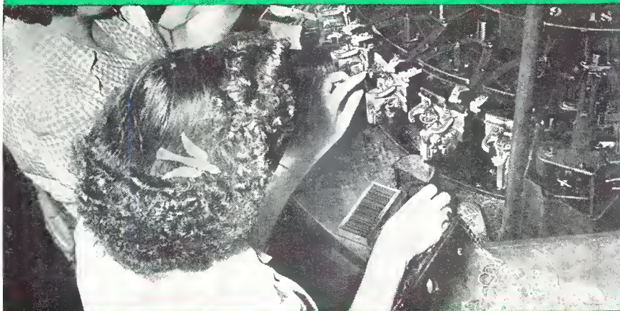
GLASS HEADERS. Small cylindrical cups of glass and metal pins are pressed into the low-loss glass base to which is joined the small glass exhaust tubing.
