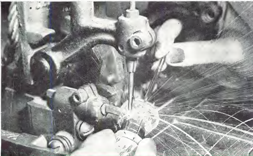
WELDING CONNECTIONS. All connections in the Lock-In Tube are welded for greater durability. Short, direct connections result in fewer joints and lower loss.
